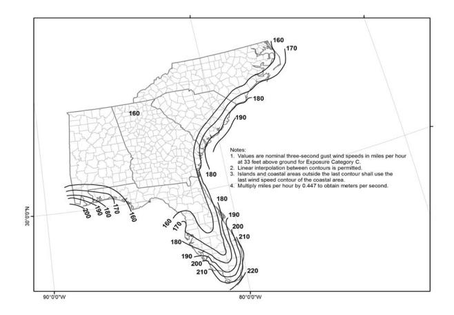
For reference purposes, Figure G-2 shows the 2010 Florida Building Code— Building design wind speed map. Figure G-3 shows the Florida Building Code— Building design wind speed with windborne debris regions.
