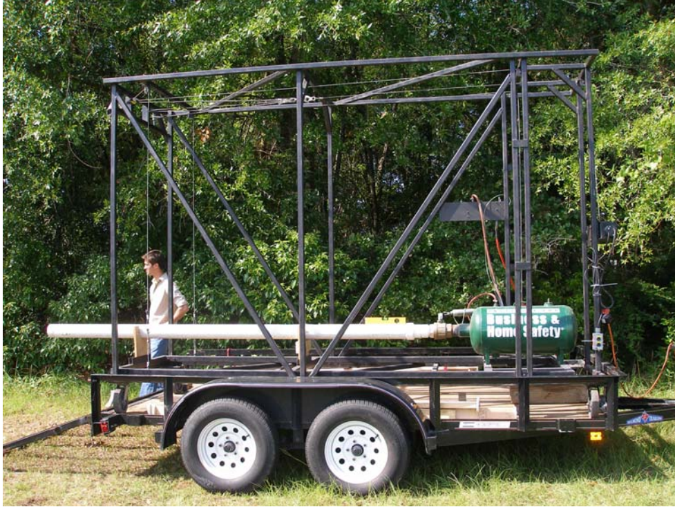
Figure 3 - Air Cannon used to Fire Missiles
