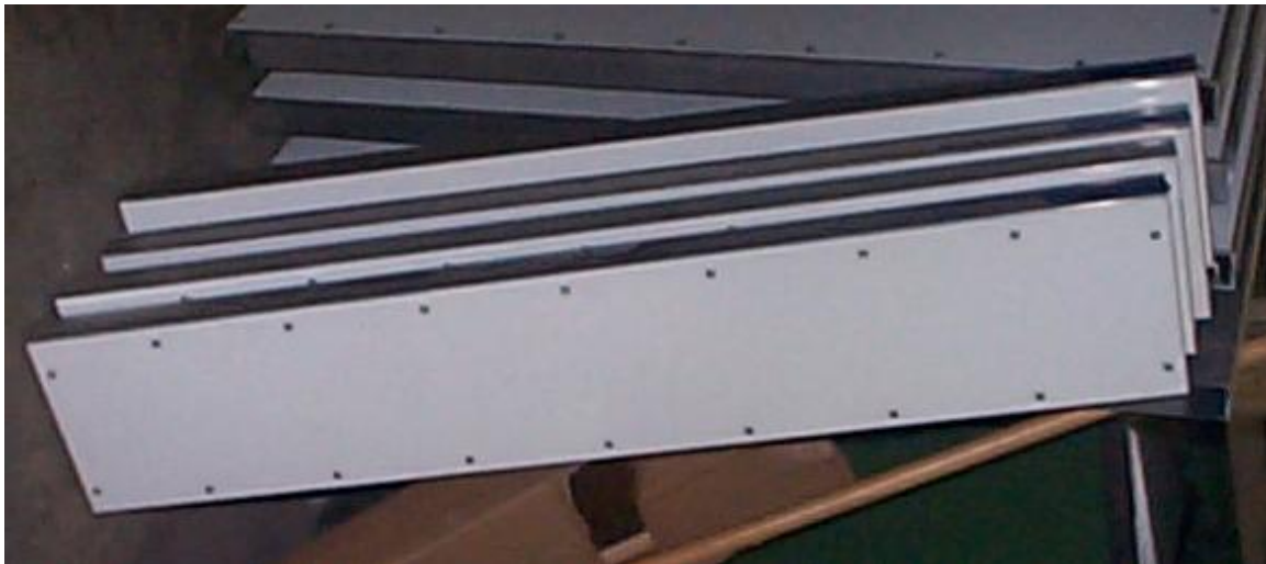
Figure 3. 4'-0" x 0'-7" Test Panel Assembled for Testing
