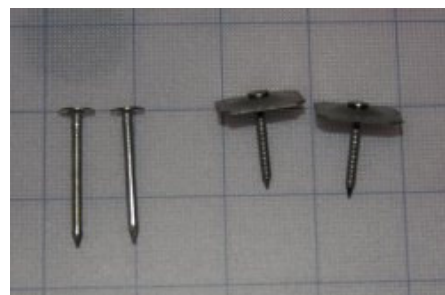
The roofing nails on the right have pre-installed plates or "tabs" to help hold the felt paper in place
