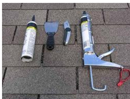
Tools and supplies needed for temporary patching of holes or to replacing torn tabs
