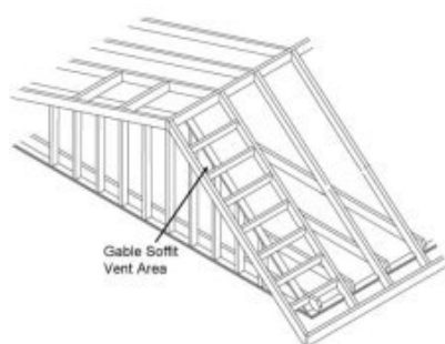
Sketch of gable roof structure with Note aluminum flashing installed and outrigger system showing water entry caulked to block water entry during point through gable soffit vent hurricane
