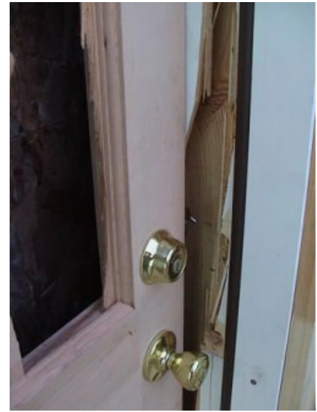
Wood panel door after impact test
