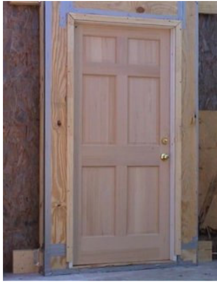
Wood panel door before impact test
