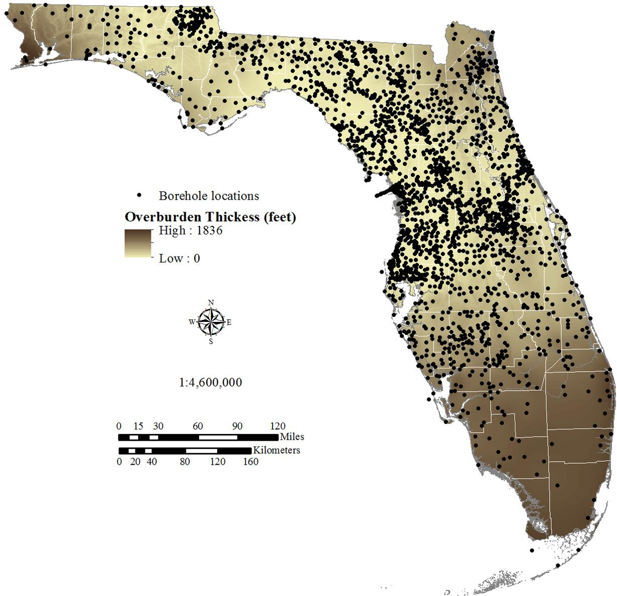
Distribution of boreholes utilized in the development of the overburden layer for the model. There were 4,269 borehole descriptions reviewed in the process of creating this layer, and 2,290 boreholes were used to create it.
