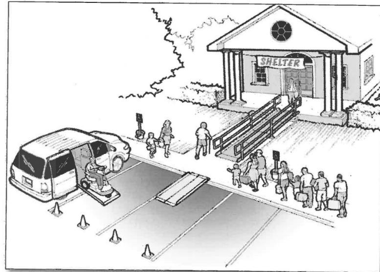
**Three standard parking spaces are converted into an accessible parking space with an access aisle. Cones mark the access aisle and a temporary curb ramp with edge protection connects to an accessible route to the shelter.**
