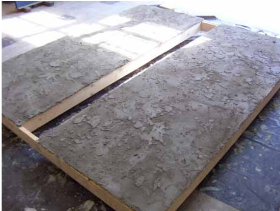
Figure 3.15: Finished Stucco over Gypsum Specimen (Upper Left) and Dinsglass Specimen (Lower Right)
