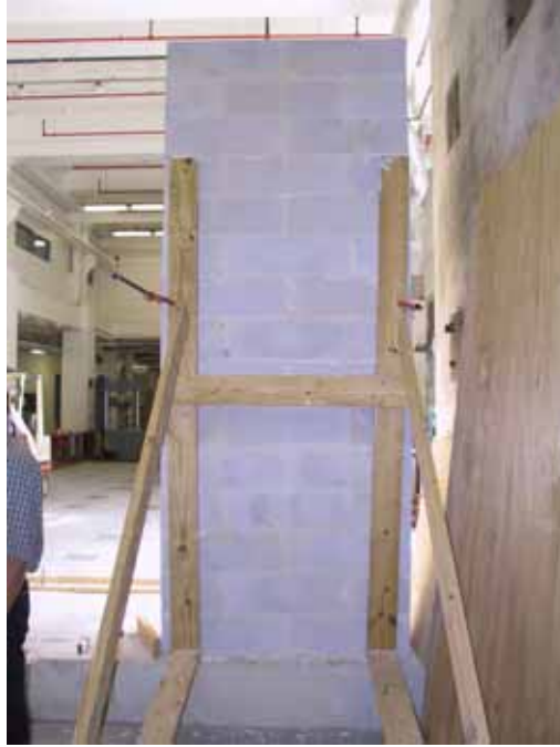
Figure 3.20: Completed AAC Specimen
