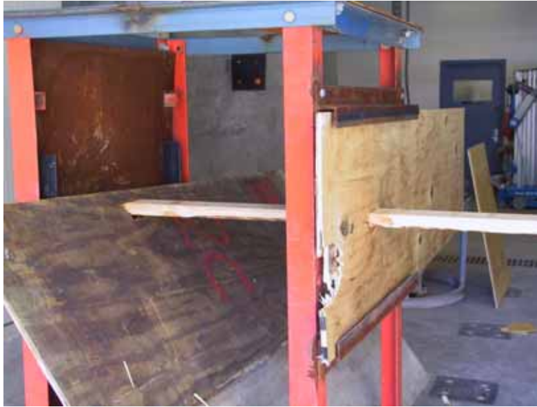
Figure 3.7: Penetration of Plywood by 15 lb Missile During Calibration
