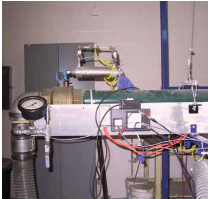
Figure 3.6: Large Missile Cannon Firing Mechanism
