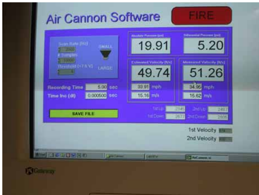
Figure 3.8: Labview Data Acquisition System
