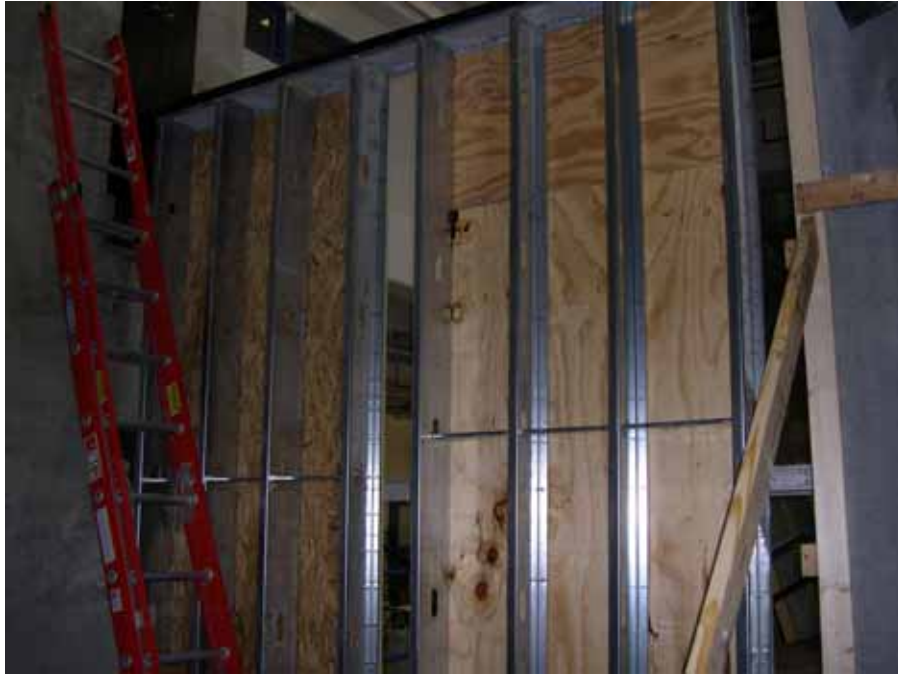
Figure 3.16: Steel Stud Wall Specimen
